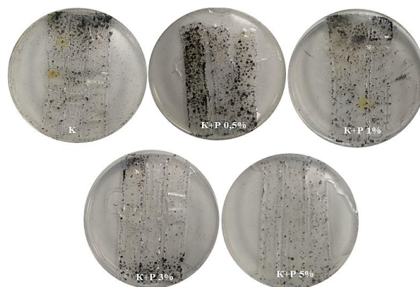
Figure 5. Fungus resistance tests of materials according to Method 1: samples obtained based on starch with different concentrations of rosemary essential oil (0.5; 1; 3; 5%)
