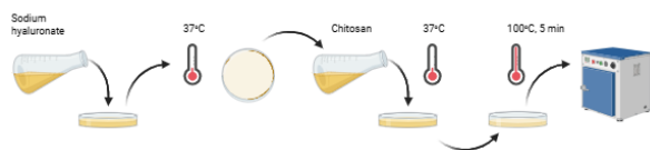
Figure 1. The process of forming a film of a polyelectrolyte complex based on sodium hyaluronate and chitosan
